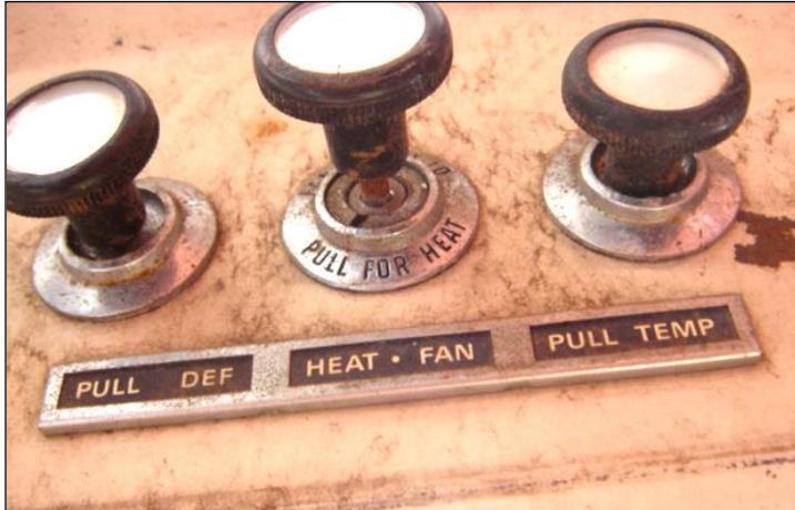
In 1973 Ford started installing label indicators between the Switches and under the Climate Controls on the dash. These labels can be seen in the picture to the left and on the **1973-1977 DASH LAYOUT** drawing on page 24. If you have a 1966-1972 dash, you can skip this step and move on to the next connection, the Gauge Cluster.
