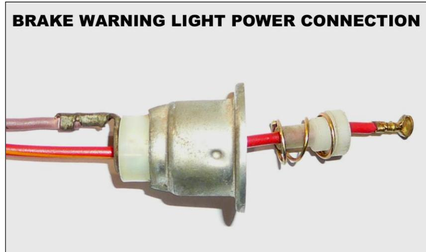
3) Install and crimp the brass contact terminal onto the wire, AVOID OVER CRIMPING. The crimpers referred to in the **RE-USING FACTORY CONNECTORS** portion of this manual, provide the best crimp.
